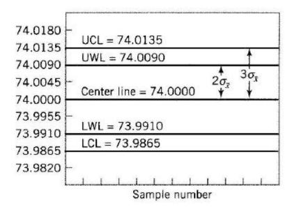
• If the process is in control, points in the *warning area* (between LWL and LCL and between UCL and UWL) are uncommon and so, with the aim of increasing the power of the chart, we stop the process if we have many points in this area.
