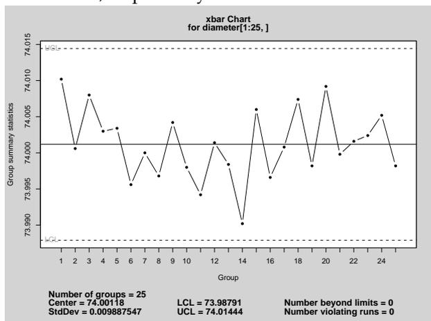
Figure 1: A  $\bar{X}$  chart for samples data.
